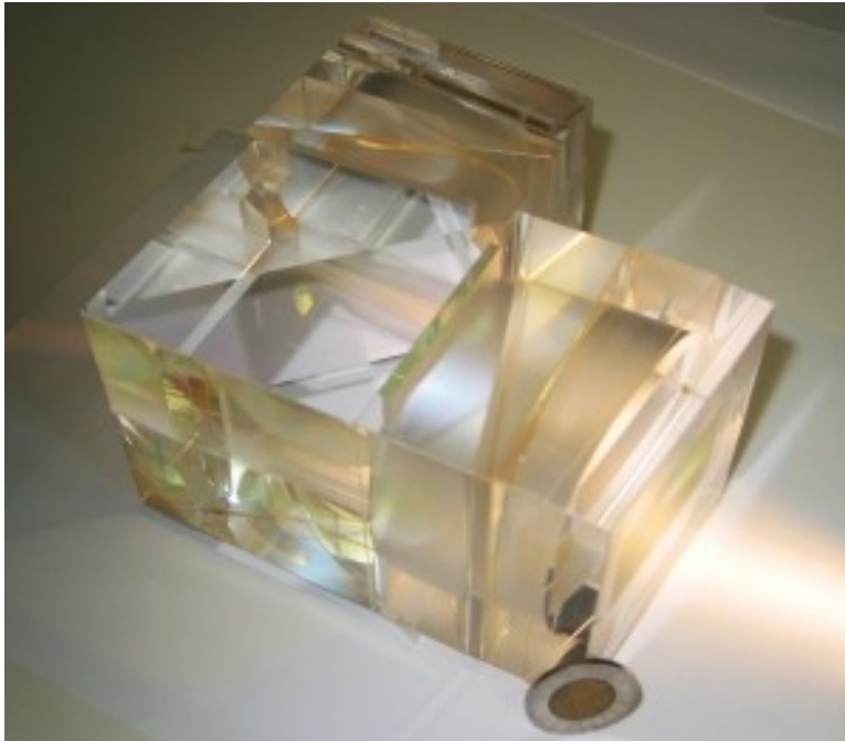
Bulk optics SHS 20 kg, 300 x 600 mm (Imaging & throughput)
